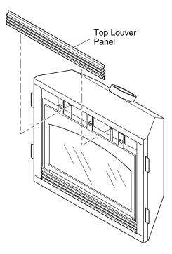
Figure 46 - Removing Top Louver Panel
